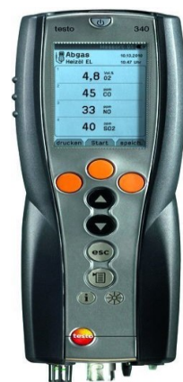
Image 4. Testo 340 flue gas analyser.
