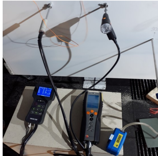
Figure 2. Test equipment, flue gas analysers 1 and 2, and aerosol and multi-gas meter (from left to right).
