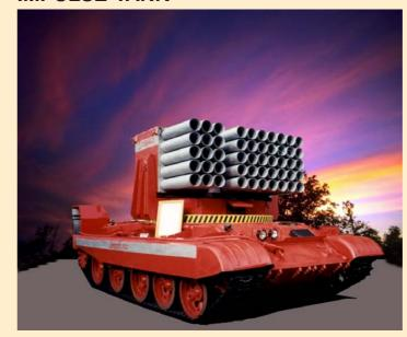
The Impulse Tank is equipped with an Impulse Storm Cassette containing 50 sprayers. It is designed for intervention in major fire accidents of the Classes A, B, C, D, E, and F. The armor shield protects its operators from the thermal radiation, chock waves, flames, explosion fragments and toxic gases.
