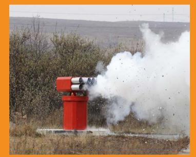
The UIS-48S modules were developed for use on fires of classes A, B, C, D, and E (depending on the extinguishing powder used) in industrial external areas. The modules are static, automated, and managed through a system with high technology sensors.
