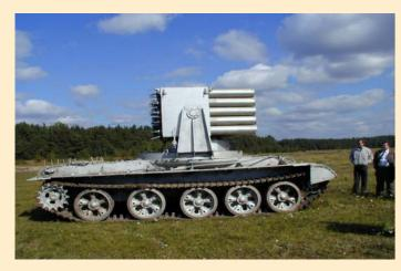
The instantaneous spraying of great quantities of extinguishing materials - denominated **Impulse Storm** - allows to efficiently extinguish fires of different classes (A, B, C, D, and E). Depending on the equipment's configuration, it is possible to spray, in less than 6 seconds, 1½ tons of extinguishing powder over a total distance of 100 meters.
