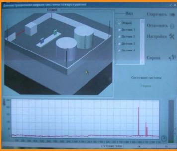
The Impulse Storm System monitors, detects and intervene upon fire detection. It is responsible for interpreting all the data received from the sensors, analyzing information, defining the strategy to be used, alarm signaling, and commanding the Impulse Storm Units (UIS).
